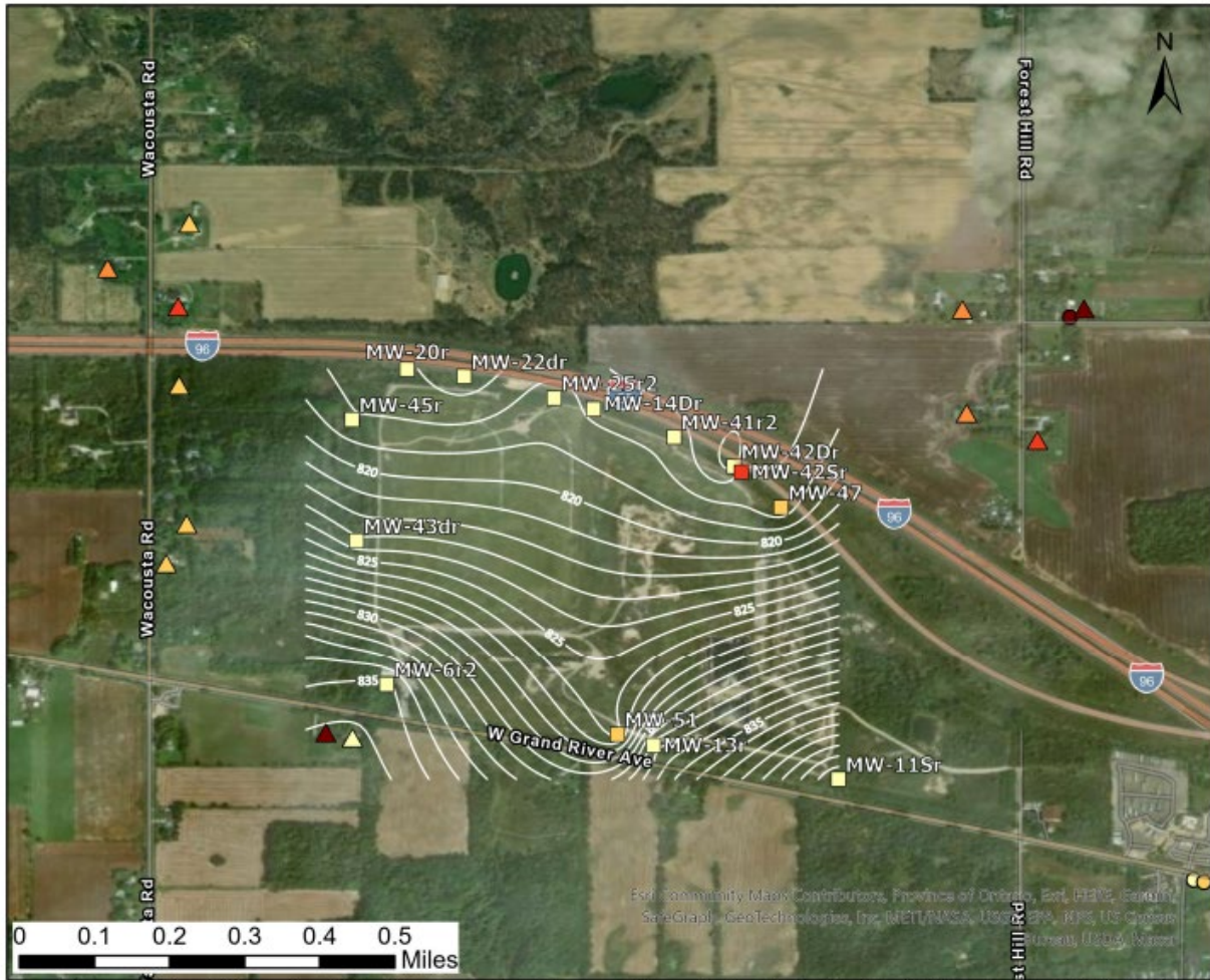
Granger Grand River Landfill - Groundwater flow and Arsenic levels in Monitor Wells, Lower Drift Aquifer (January, 2023 sampling) and Private wells (June 2023 sampling)
